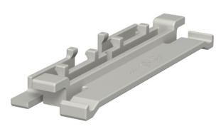
Cover clip for better and easier laying of lines in the WDK trunking. The cover fixing device can be moved along the entire length of the trunking. The cover clip is locked on one side and moved forward. This provides a 30° opening, meaning that cable routing is very simple. From trunking widths of 110 mm, the cover clips can also be used as a mounting aid.
