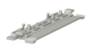
Cover clip for better and easier laying of lines in the WDK trunking. The cover fixing device can be moved along the entire length of the trunking. The cover clip is locked on one side and moved forward. This provides a 30° opening, meaning that cable routing is very simple.
