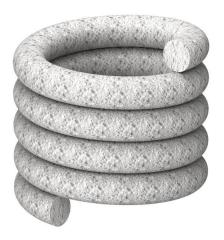
The noise limit barrier is used to reduce the transmission of airborne noise, e.g. when the trunking system is run through a wall between two offices. The noise limit barrier is made of glass wool, which, when delivered, has a diameter of approx. 30 mm. The goods sold by the metre are delivered in a box, the length of the material is 50 m. The material need not be greatly compressed during mounting.
