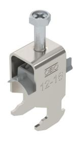
Clamp clip with hammerhead foot, plastic pressure sleeve made of polypropylene. For vertical and horizontal mounting of 1 single cable on a C-profile rail. For a slot width 16–17 mm. With 1-start screw thread on pressure sleeve, universal hexagonal screw head WAF10, with slot and cross recess. Suitable for assembly indoors and outdoors. We recommend the use of a counter-sleeve.
