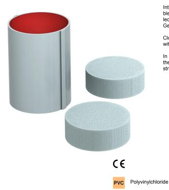
Internally coated pipe shells with click lock. The inner space can be fitted with cables and electrical installation pipes completely. For interior application. CE-labelled, European approved construction product according to ETA-13/0904 and German general type approval. Fire resistance up to 120 minutes.
