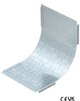
Cover for all rising vertical bends. The fastening is guaranteed by the overlap of the cable tray covers. The cover can also be fastened using cover clamps.
