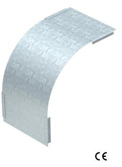
Cover for falling vertical bends of side height 35 mm. The fastening is guaranteed by the overlap of the cable tray covers. The cover can also be fastened using cover clamps.
