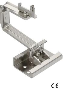
Roof hook to mount photovoltaic modules on pitched roofs in combination with the TP 45 support profile. Suitable for tiled roofs. Lockable fastening on support profile. Mounting on rafters with TKS wafer-head screws. Roof hook can be infinitely adjusted horizontally and vertically using glands, correct spanner Torx 40. Height adjustment in the range of the roof slat between 40-54 mm, side adjustment option up to 76 mm, height adjustment of the support profile up to 18 mm.
