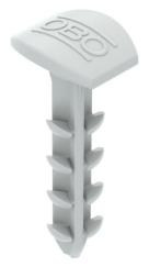
Push-fit plug Delta-Push® for mounting electrical installations. Suitable for concrete, calcareous limestone, full brick, hollow brick and porous concrete. Tooless mounting by pushing into a drill hole in a wall or on a ceiling. Without screws. To install cable trunking or labelling panels, for example.
