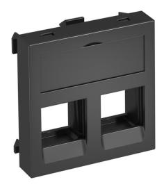
Data technology support with straight outlet and without a locking slider to accept two data technology connection modules with RJ45 socket. The locking fastening is suitable for horizontal and vertical installation in the system environment. Type C has a mounting opening of 19.30 x 14.80 mm and is designed for direct fastening of the data connection modules in the mounting opening.
