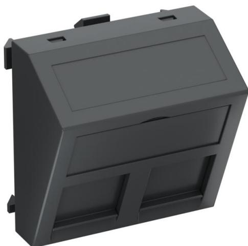
Data technology support with slanting outlet and locking slider to accept two data technology connection modules with RJ45 socket. The locking fastening is suitable for horizontal and vertical installation in the system environment. Type F has a special module seat and is designed for indirect fastening of the data connection modules in the mounting opening.
