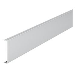
Aluminium cover, for closing Rapid GA device installation trunking and ISS service poles with a 76.5 mm system opening. The firm position of the cover and electrical contact to the lower part of the trunking and service pole is guaranteed thanks to type RKV3V locking brackets. There are 6 pre-mounted locking brackets included per delivery length (2,000 mm).
