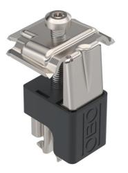
Universal clamp to mount photovoltaic modules on flat and pitched roofs, suitable as a clamp between 2 modules or as an end clamp. Lockable pre-fastening on TP 45 support profile and on STK and STL supports. Suitable for 10 mm slot width. Can be rotated through 90° after engaging. Lockable fastening of the PV module with Torx 30 wrench.
