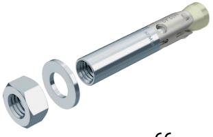
Bolt tie BZ-IG with internal thread for the anchoring of medium-duty to heavy-duty loads, both in cracked and non-cracked concrete. It combines high approved loads with small edge distances and axial spacings. Undercutting the drill holes is not necessary.
