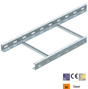
Cable ladder with perforated side rail of side height 45 mm with riveted C profile rungs, open in an upwards direction.
