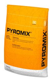
Mortar to create cable and combination insulation in solid walls and ceilings. Suitable for pumping, pressing and for manual installation. Adding approx. 6 litres of water to 20 kg of dry mortar produces about 20 litres of workable compound. For interior application.
