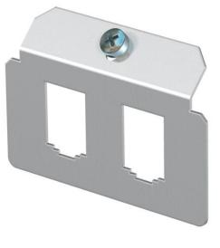
Support plate to accept two connection modules for data connection modules of the following types BTR: E-DAT;Dätwyler: MS and MS-N; Kerpen: VarioKeystone.
