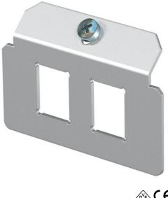
Support plate to accept two data connection modules of the following types: Brand-Rex: shielded; EKU: E-Stone; Dätwyler: KS-T, MS-K and KU-T module; R&M: Snap-In and Keystone; Rutenbeck: UM and UMflex; SETEC: MKJ, UKJ and XKJ; Siemon TERA; Telegärtner: AMJ and UMJ; 3M: CAT6 and CAT6A. Dimensions of a mounting opening in mm: 19.30 x 14.80.
