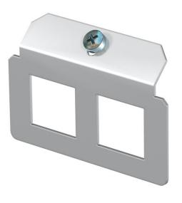
Support plate to accept two data connection sockets, type Panduit in combination with Panduit adapter CMNZABL-X or CMNZAWH-X. Dimensions of a mounting opening in mm: 19.8 x 21.2.
