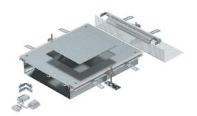
Ready-to-mount trunking extension unit with a device installation lid for the installation of a flush-mount unit of nominal size 9, consisting of the trunking base (floor trough with side and floor covering contact profiles), trunking lid with blank mounting opening and a flushfloor end cover. The scope of delivery contains 3 height-adjustable fixing brackets, 3 screed anchors, 1 lid butt support and 1 construction set for 90° angle
