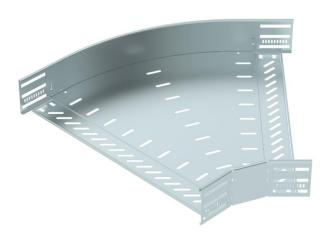
45° bend for the creation of a horizontal branch, fitting for lock and screw-on cable trays of side height 85 mm. Screwless mounting with double clamps or screw connection with FRS truss-head screws and M6 combination nuts. Can be used in indoor areas. Fastening material must be ordered separately.
