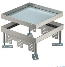
"Blank" height-adjustable cassette for the creation of an inspection opening of nominal size 4. Installation of devices in duct systems, raised and cavity floors in interior dry or wet-care floors. Only suitable for smooth floor coverings. For the installation of three UT4 universal supports for nine single devices with support ring/support clamp or 12 Modul 45® devices. 3 APMT5 cover plates can be installed.
