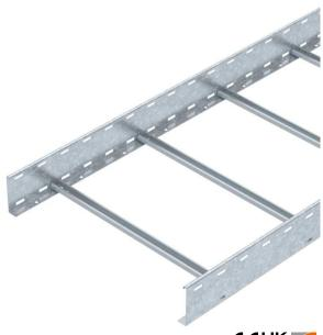
Cable ladder with 110 mm side height with welded C30 profile rungs which are open in an upwards direction. Rolled side rail for reinforcement and as edge protection. Fastening to the bracket takes place using clamps, type LKS 40. The slot dimension of the frame is 16.5 mm and the appropriate U clamp clip is type 2056
