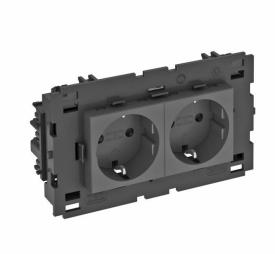
Protective contact socket with connection to side, double 0°, with increased touch protection, with screwless terminals, 2-pin, 16 A, 250 V~, with connection terminals to IEC 60884-1, suitable for the installation in Rapid 80 device installation trunking systems.
