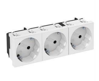
Protective contact socket triple 33°, with increased touch protection, with screwless terminals, 2-pin, 16 A, 250 V~, with connection terminals to IEC 60884-1.
