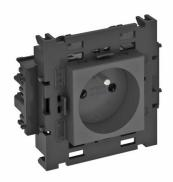
Earthing pin socket with connection to side, Single  $0^\circ$ , with increased touch protection, with screwless terminals, 2-pin, 16 A, 250 V $\sim$ , with connection terminals to IEC 60884-1, suitable for the installation in Rapid 80 device installation trunking systems.
