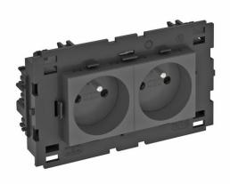
Socket with earthing pin with side connection Double  $0^\circ$ , with increased touch protection with screwless terminals, 2-pin, 16 A, 250 V $^\circ$ , with connection terminals to IEC 60884-1, suitable for installation in Rapid 80 device installation trunking systems.
