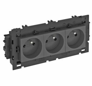
Earthing pin socket with connection to side, Triple 0°, with increased touch protection, with screwless terminals, 2-pin, 16 A, 250 V~, with connection terminals to IEC 60884-1, suitable for the installation in Rapid 80 device installation trunking systems.
