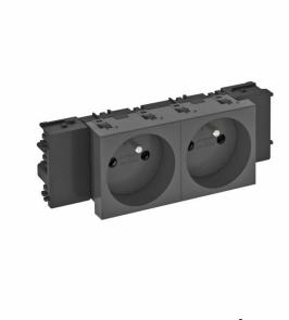
Earthing pin socket with connection to side, Double 0°, with increased touch protection, with screwless terminals, 2-pin, 16 A, 250 V~, with connection terminals to IEC 60884-1, suitable for the installation in Rapid 45 device installation trunking systems.
