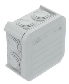
Junction box for the connection of cables and lines indoors and in protected outdoor areas. Square design with plug-in seals to the sides and knock-out entries in the bottom. Suitable for wall and ceiling mounting and on mounting panels. With the option to fasten inside. With fixed clamping cover. Flame-resistant type made from special polypropylene.
