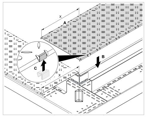
Fig. 21: Mounting the cover on a corner connection
