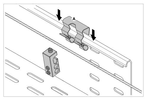
Fig. 13: Mounting the clamp spring
