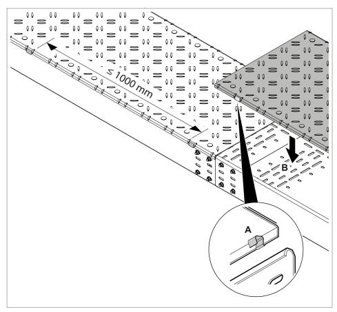
Fig. 18: Mounting the cover, type DBKR, with cover clamps
