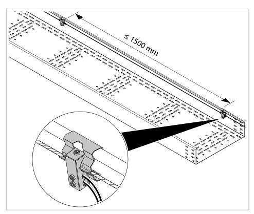
Fig. 12: Spacing of clamp springs with connection terminal
