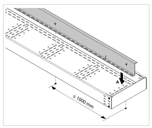
Fig. 11: Barrier strip mounting
