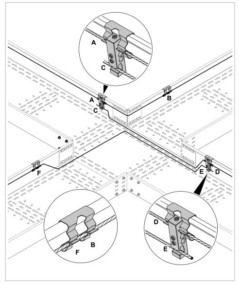
Fig. 16: Mounting of conductor cross-over, double connection terminal
