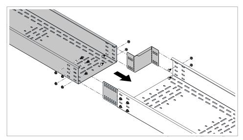
Fig. 9: Changing the cable tray width
