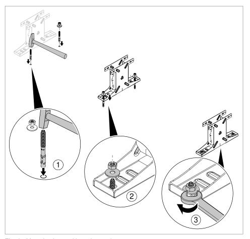
Fig. 3: Mounting base with wedge anchors
