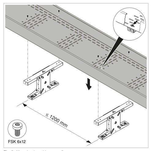
Fig. 5: Mounting the cable tray on floor supports
