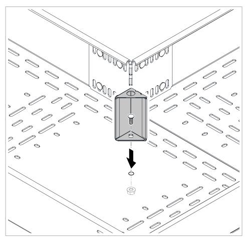
Fig. 17: Installation of cover support
