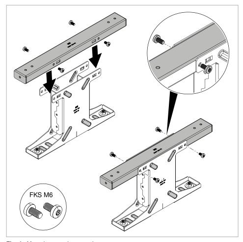
Fig. 4: Mounting crossbeam on base
