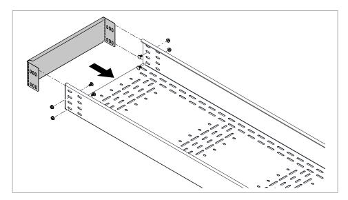
Fig. 10: Closure of open ends
