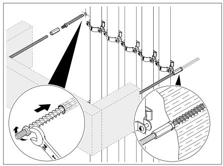
Fig. 11: Fastening threaded rods on the wall
