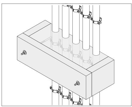
Fig. 1: ZSE90-.../ZSE90-...L strain relief for cable installation with cable spacer clips
