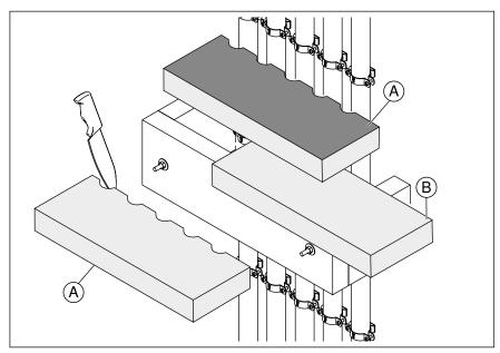
Fig. 19: Filling the housing
