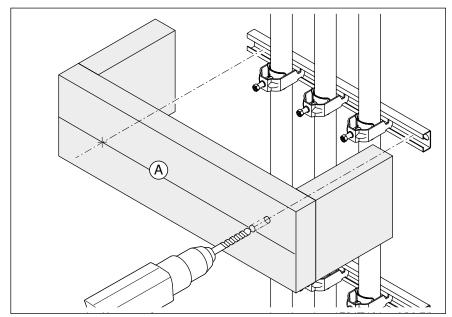
Fig. 10: Pre-drilling the housing
