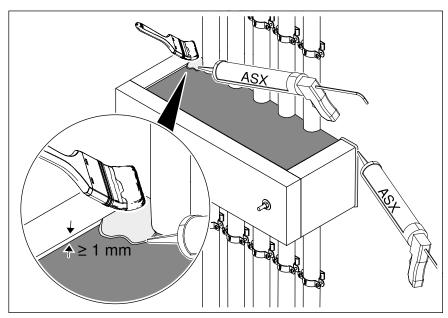
Fig. 20: Sealing with fire protection filler
