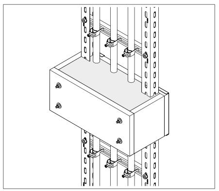
Fig. 26: Fully mounted strain relief on suspended vertical ladder
