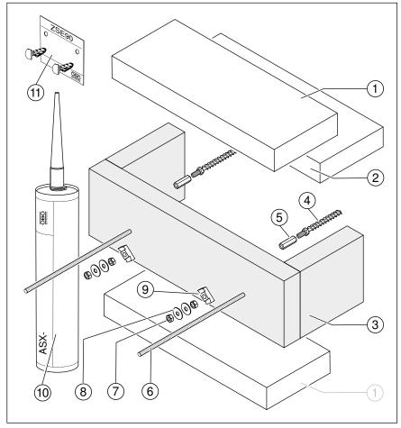
Fig. 5: System components, housing, type ZSE90-...
