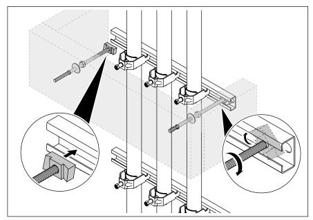
Fig. 13: Fastening threaded rods using slide nuts
