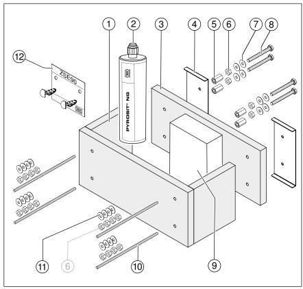
Fig. 7: System components, housing, type ZSE90-...LH
