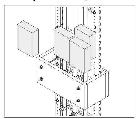
Variant A: Filling with foam blocks and fire protection foam
