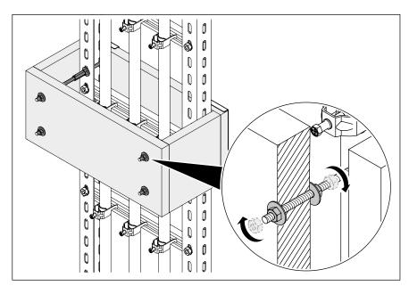
Fig. 18: Housing fastened on threaded rods
