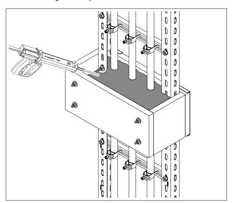
Fig. 25: Filling the housing with fire protection foam
