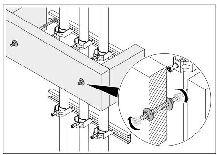
Fig. 14: Fastening the housing on threaded rods
