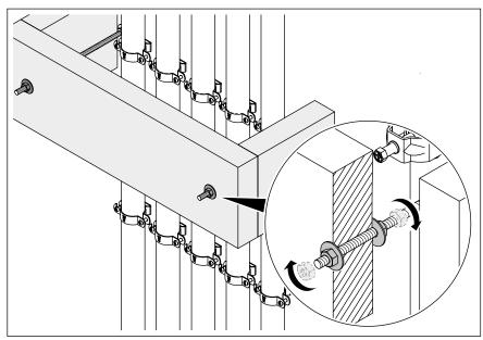
Fig. 12: Fastening the housing on threaded rods
