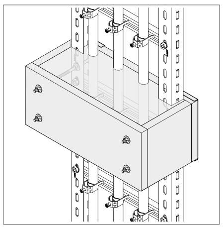
**Fig. 4:** ZSE90-... LH strain relief for cable installation on suspended vertical ladder
