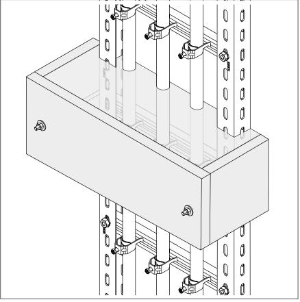
Fig. 3: ZSE90.../ZSE90-...L strain relief for cable installation on vertical ladders on the wall
