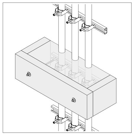
Fig. 2: ZSE90-.../ZSE90-...L strain relief for cable installation on profile rail
