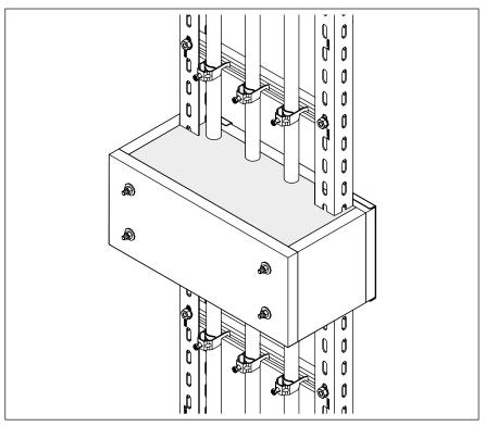
Fig. 24: Fully mounted strain relief on suspended vertical ladder
