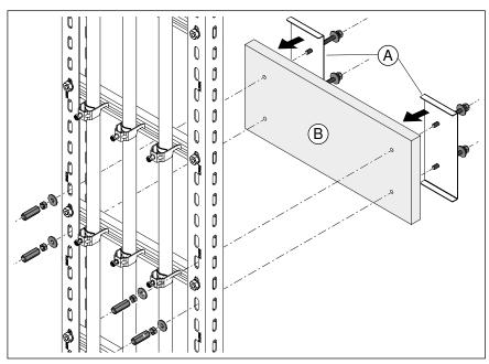
Fig. 15: Connecting the back plate to lock plates
