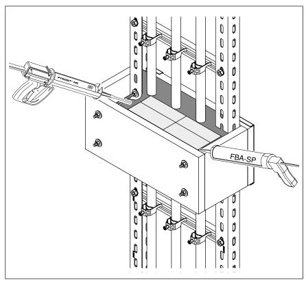
Fig. 23: Applying fire protection foam.
