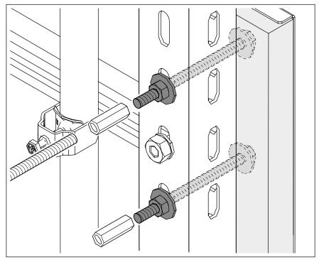
Fig. 16: Fastening the back plate to vertical ladder rails with lock plates
