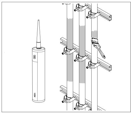
Fig. 9: Coating cables with fire protection filler
