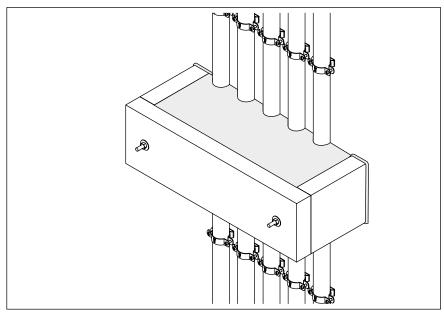
Fig. 21: Fully mounted strain relief
